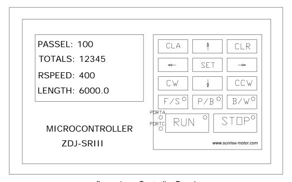
figure 1. Controller Panel
